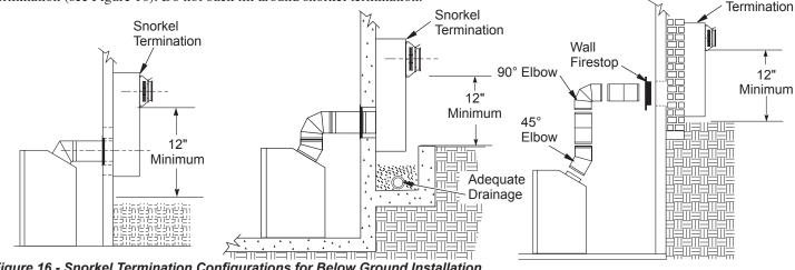
Figure 16 - Snorkel Termination Configurations for Below Ground Installation
